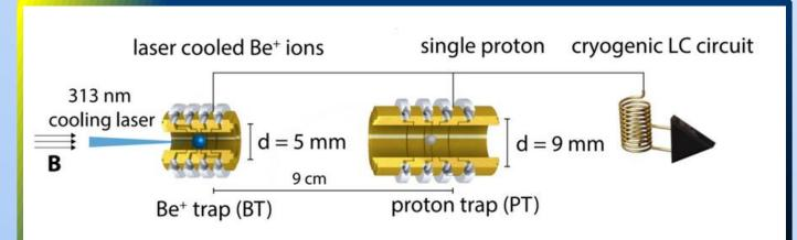
Sympathetic laser cooling system using a single proton, a cloud of laser cooled beryllium ions and a cryogenic LC circuit to transmit the cooling power by image currents
